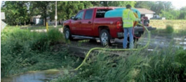
20 foot bottom fill kit included for refilling tank from any nearby water source for fast action.
